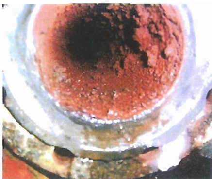
Scale before Hydroflow water conditioning
