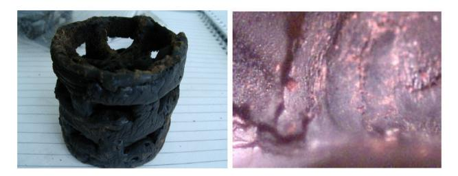
Around the perimeter of the tower some packing exhibited deposits that are clearly not carbonate. It appeared that some low temperature melting material had settled on to the packing.
