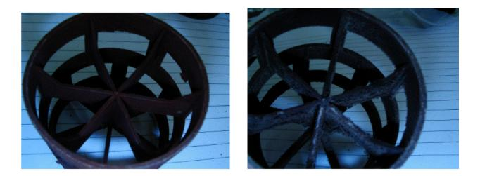
In the 2nd level, the packing was clear of crystals as all the loose crystals washed off.
