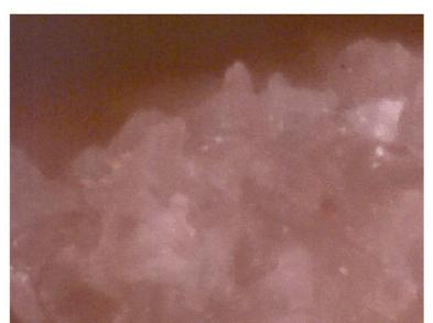
A microscope enlargement clearly shows the individual calcite crystals.
