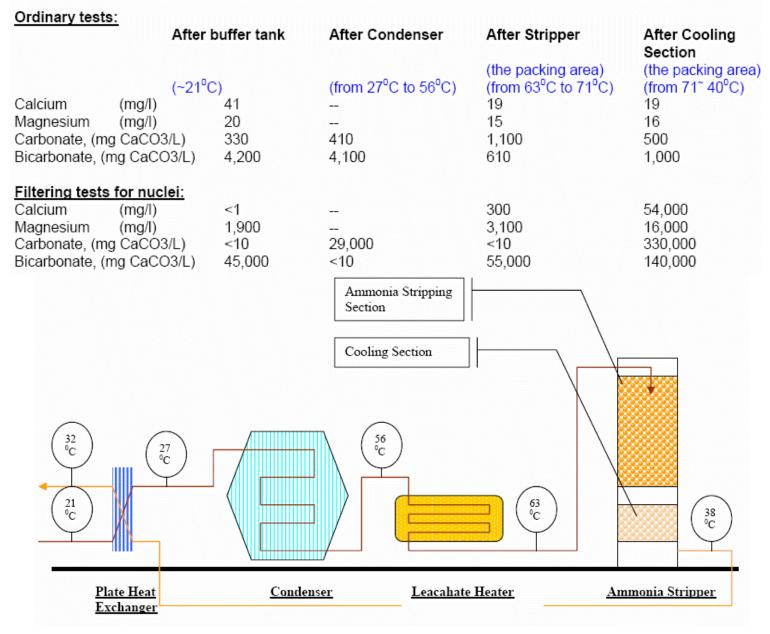
Tseung Kwan O Landfills have been fitted with Hydropath technology to minimize maintenance work on the ammonia-stripping tower and to maintain the heat exchangers efficiency.
