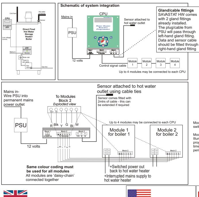
Each CPU has to be configured for number of boilers/modules. Place jumper as follows - Jumper not installed (factory default) 1 module. Position 1 (far left) 2 modules. Position 2 (middle) 3 modules. Position 3 (far right) 4 modules.
