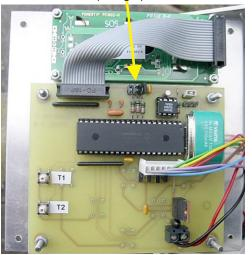
Each module has to be configured for it's position in order. Place jumper to suit each module i.e. Position 1 for module1 (default setting) Position 2 for boiler/module 2 etc.
