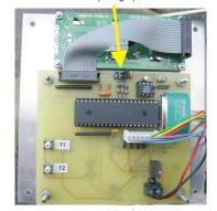
Each module has to be configured for it's position in order. Place jumper to suit each module i.e. Position 1 for module1 (default setting) Position 2 for boiler/module 2 etc.
